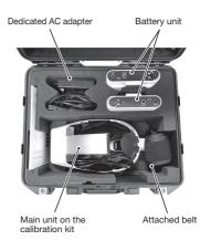
\*Match the orientation of the main unit with that in the illustration affixed to the calibration kit.
