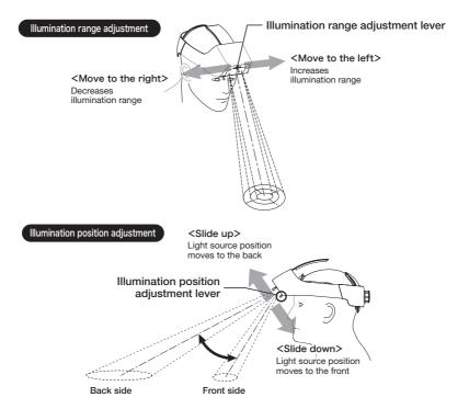
The optimal illumination position depends on the operation.
